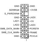
This connector supports Trusted Platform Module (TPM) system, which can securely store keys, digital certificates, passwords, and data. A TPM system also helps enhance network security, protects digital identities, and ensures platform integrity.
